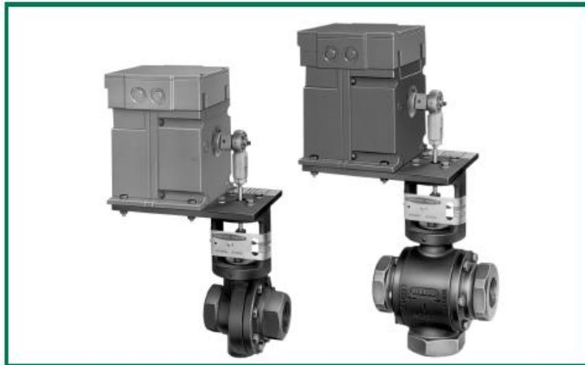
A selection of control valves featuring the Jordan sliding gate seat and heavy-duty industrial motors for proportional (resistance), on-off, or 4-20 mA electronic control. Models include the Mark 33 in sizes 1/4" through 2", the high flow Mark 331/332 with Cv's up to 70, and the Mark 39 with three-way body.
